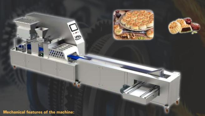
The machine operates six three-phase motors of the original brand in Turkey, capacitive and optical sensors, German-made, Zic, Italian and German-made air group, Festo – Metal Work – touch screen / 7 / inch with its own electronic brain Delta The machine is made of food chromium by 85%, and coated With a high-end stainless steel cover designated for this purpose. Electricity / 3 / kilowatt 7 / Hz / 50-60 / Volt / 220
