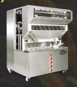
The covers are designed as glass so that the movements of the dough inside the machine can be observed more easily. The machine can be easily moved to the desired location thanks to the wheels underneath. The dough capacity of the machine is 154 and 238, and the resting capacity is 1800-2000 pieces per hour.
